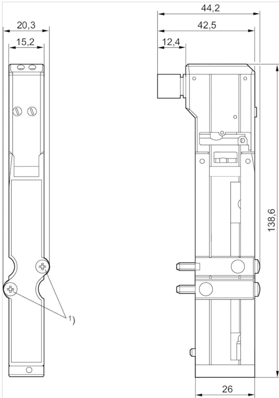
1) Mounting screw: X-slot DIN EN ISO 4757-Z1tightening torque for mounting screw [Nm]: 1.3
