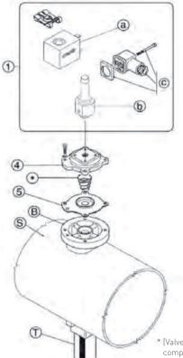
\* [Valve Body(B) + Tank(S) + Valve blowpipe (T) are to be considered single and complete module.] (No spare parts available for this configuration.)
